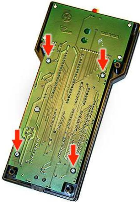
2 Remove the 4 screws holding the printed circuit board to the case.
