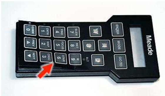
4. Peel the old keypad from the case. It may be easiest to start with a knife or flat-head screwdriver, inserting it between the keypad and the case along the right side near the #6 button, and prying the edge of the keypad up.
