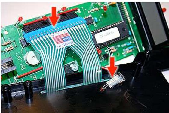
3 Flip the PCB over and remove the LED connector and the keypad connector. Disconnecting the keypad may take some effort--be sure to pull straight to avoid bending the pins.
