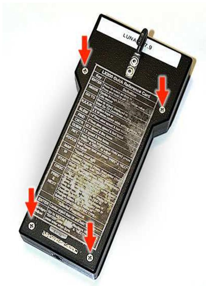
1. Remove the 4 flat-head screws from the back of the controller.
